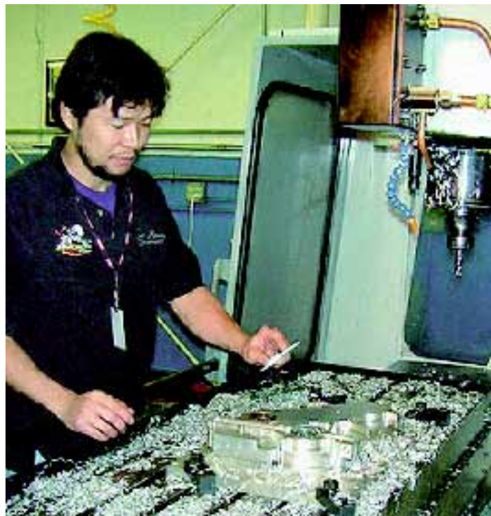
Nobu Okawa reviews the imported solid model of the transfer case housing and cover before beginning the Mastercam toolpathing process.
