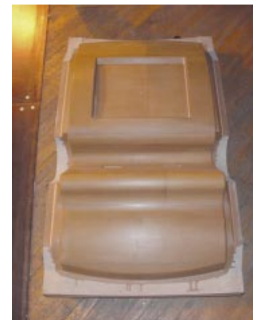
The ATM front panel mold is now complete — finish-cut and sealed — and ready to be mounted for production vacuum forming.
