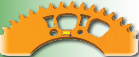
Create a pattern of solid features and create multiple copies on a part.
