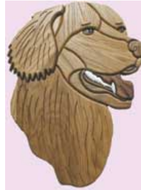
Golden Retriever, from among WoodenNature's stock breeds, is reproduced from stored Mastercam toolpaths. If the design is changed, the associative toolpaths regenerate with the click of a mouse button.
