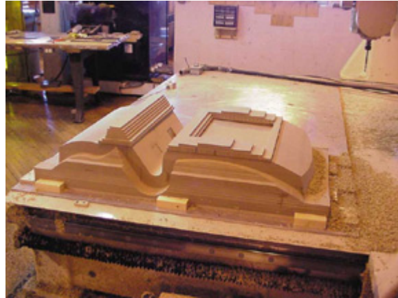
RenShape blocks have been added to the Mastercam-machined third layer prior to roughing. Each layer has been cut to precise boundaries and is ready to accept the bottom plane of the next.
