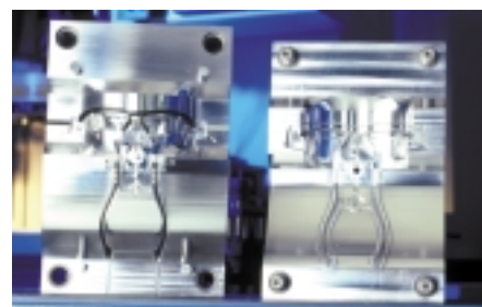
Figure 7 The customer's requirement that this mold for well-known sunglasses be self-ejecting validated the choice that RoMold — a Rochester, NY moldmaker — made to go five-axis. The complex mechanism, moving undercut mold elements, demanded five-axis machining.
