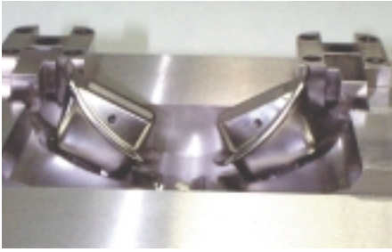
Figure 8 With the eye-hole ejection section fully extended, it's easy to understand the extensive five-axis undercutting necessary to produce these mold parts.
